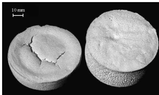
Fig. 6. Samples gelled after crosslinking of PVAI (left) and using gelatin (right).
